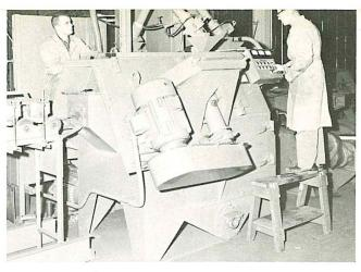
Senior Tester Truman Wesco and Assistant Tommy Thompson, behind the Wheelabrator, prepare a 3-wheel rod cleaning machine for Eaton Manufacturing Company's demonstration. The Ohio firm sent us 67 coils of wire rod in order to make a comparison between Wheelabrator descaling and their present acid pickling operation.
